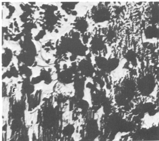
Figure 2 Semi-continuous flakes of M_6C , extracted from an intergranular fracture ( \times 5250 ).
